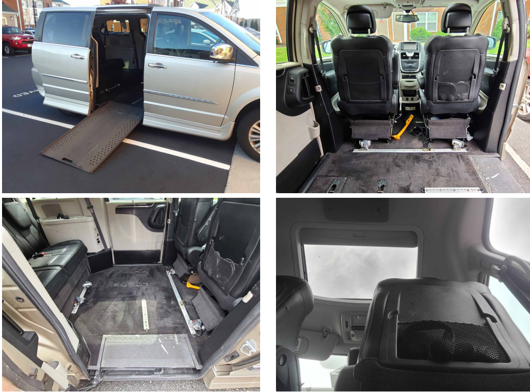
Figure 2. Photos of the 2015 handicapped-accessible Chrysler Town & Country minivan modified by Rollx Vans used in this study showing the motorized ramp, the cargo area (for the power wheelchair base), and the automated sunroof.
